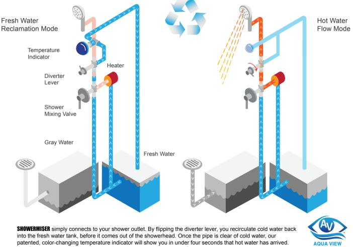
Just flip the diverter lever back to the showerhead and hot water will flow.
